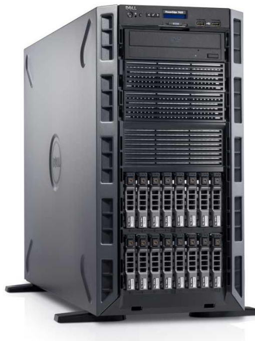
Figure 1. Front view 16-drive bay without bezel
